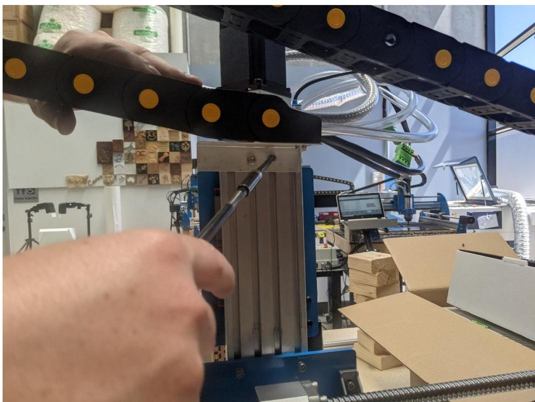
Move the drag chain down and twist the left hand side up. Tighten the bolts to secure in place.
